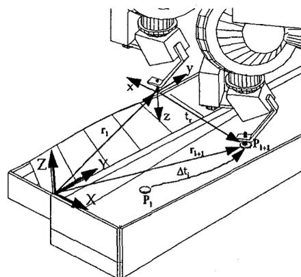
Fig. 2 Relationship between the moving object and gripper
