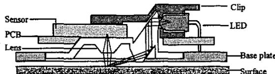
Figure 5 Assembly view illustrating the principle
