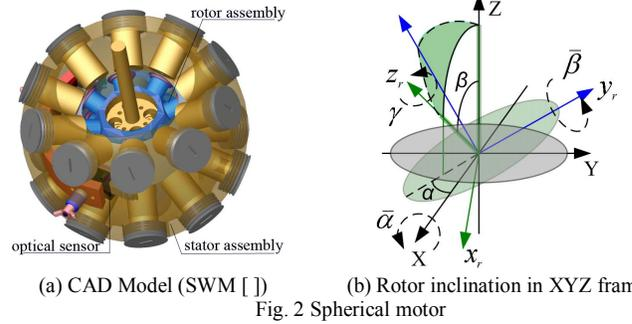
Fig. 2 Spherical motor
