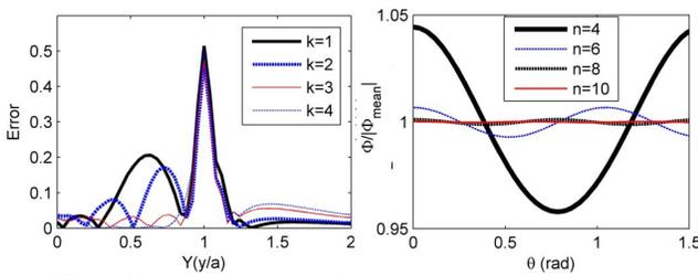
Fig. 5 Effect of  $n$  and  $k$  on modeling errors of PM with  $\gamma(2a/\ell) = 1$
