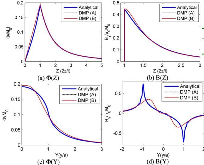
Fig. 4 Potential and flux density along Y and Z axes ( $n=6$  and  $k=1$ )
