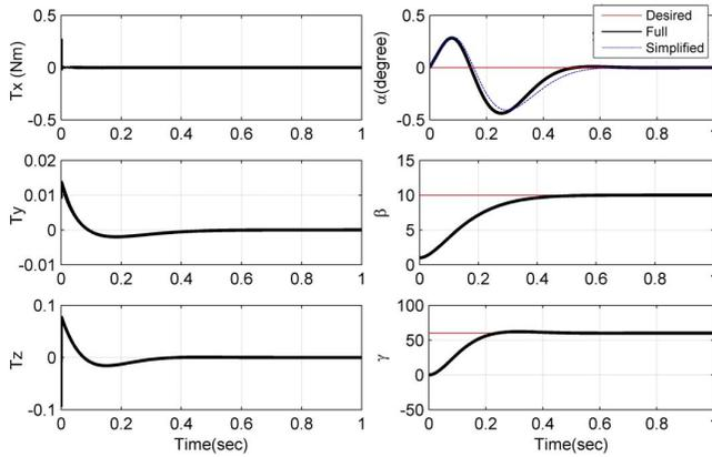
Fig. 8 Step response of Spherical Motor (Design B)
