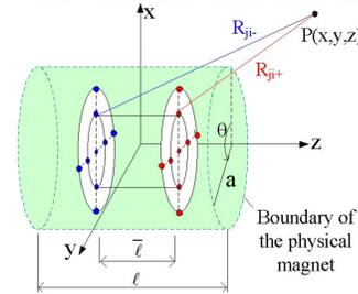
Fig. 1 DMP model of a cylindrical magnet
