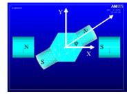
(a) Torque computation between a PM and an EM pole-pairs
