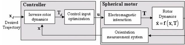
Fig. 3 Closed-loop control of the spherical motor
