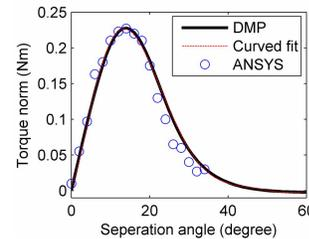
Fig. 7 Torque between a PM pole-pair and an EM pole-pair
