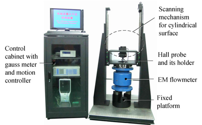
(a) Dry calibration setup
