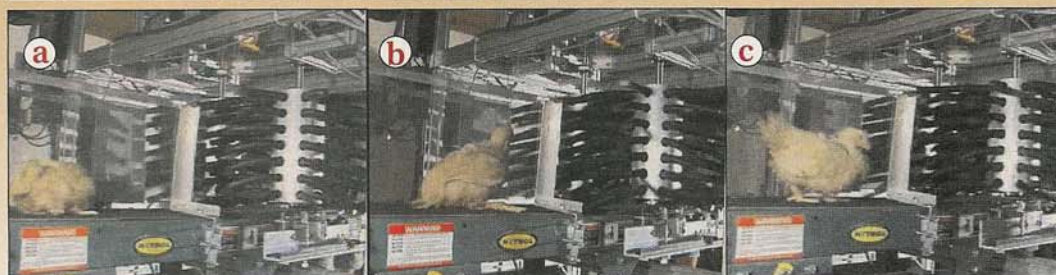
Figure 4. Typical bird posture on approach to the compliant grasper (a) sit down (b) sit up (c) stand
