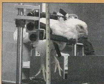
Figure 5. Mechanical hand and sideview of the compliant grasping of a broiler
