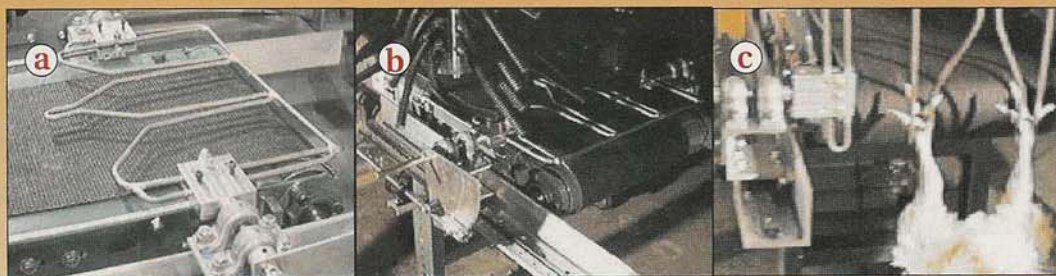
Figure 3. Prototype shackle used with the compliant grasper (a) prototype shackle and inversion system; (b) shackle positioned under compliant grasper; (c) bird hung on rotated shackle
