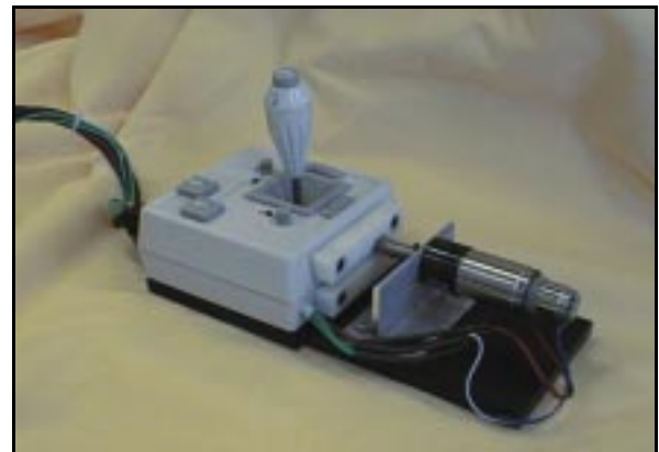
Figure 8 Prototype active joystick
