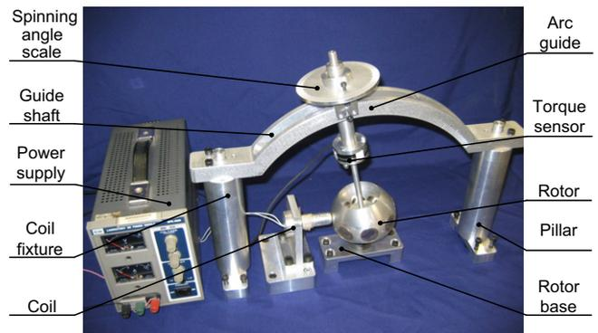
Fig. 7. Testbed for force/torque measurement of single coil.
